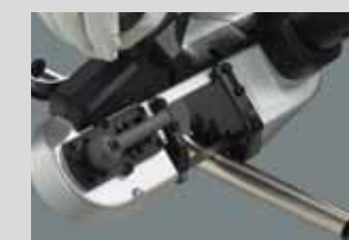
Blade speed 1 (low speed) For cutting stainless steel stock, etc.*2
